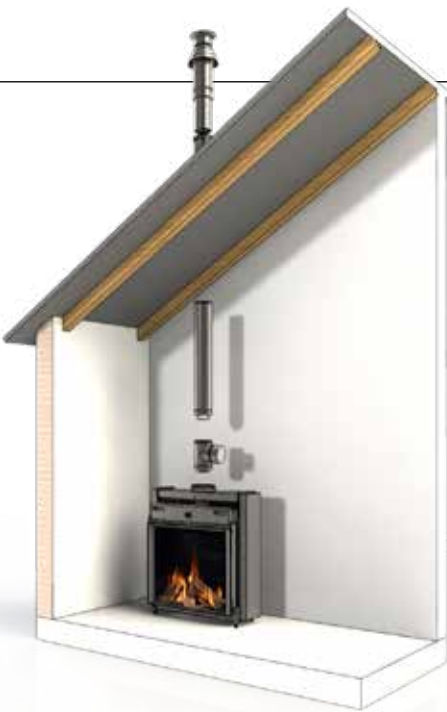
Via the roof (inclined) • direct or with the pipe bends
