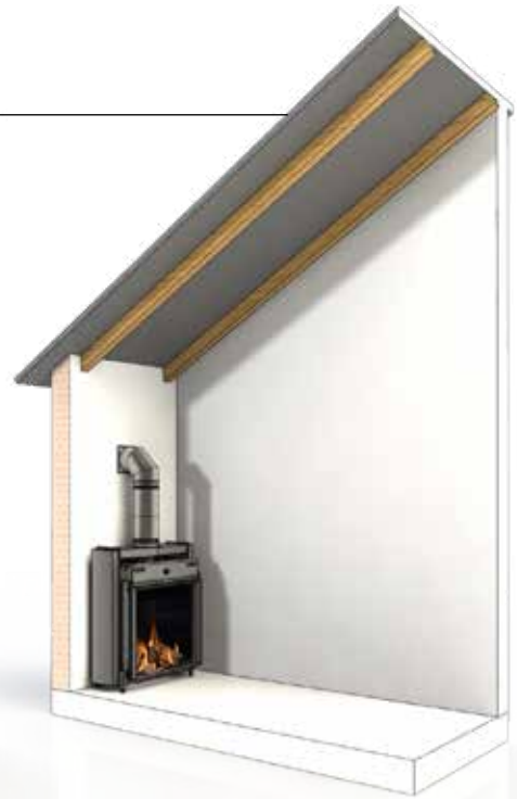
Via the outer wall • first metre is vertical, followed by a 90° pipe bend
